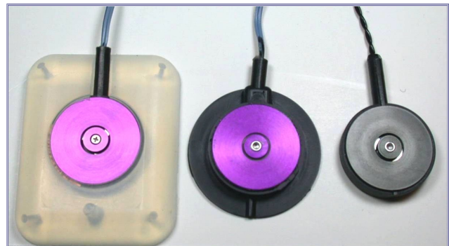
From left: C-2 Tactor with Silicone Gel “snap-in” mounting pad; C-2 Tactor with integral polyurethane flange for sewing into a garment; ruggedized C2-A Tactor with internal moisture/sand seal and highly flexible “tinsel” wire with Kevlar strength member.
